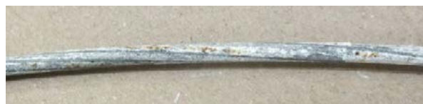
Figure 28: Rust observed on steel core strand
