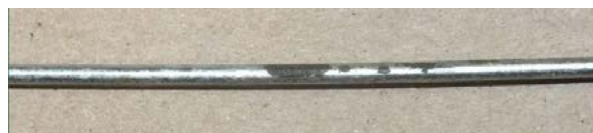
Figure 27: Degradation of galvanic zinc coating
