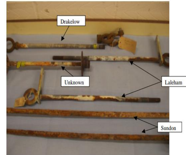
Corroded through-bolt failure
