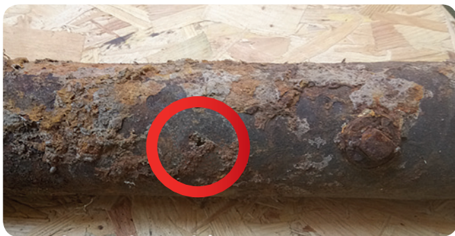
4" cast iron pipe showing damage
