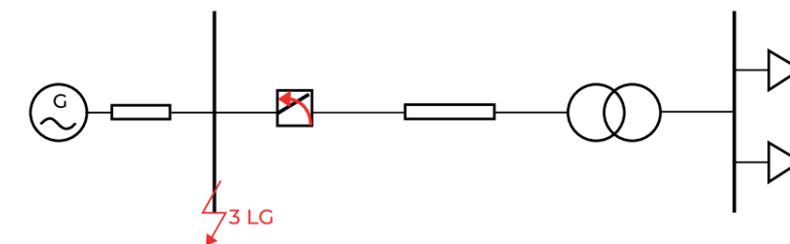
Figure 2: Simple circuit diagram showing a fault
