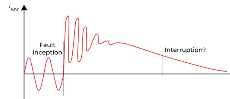
Figure 5: Graphical representation of current flowing as a result of fault in Figure 4
