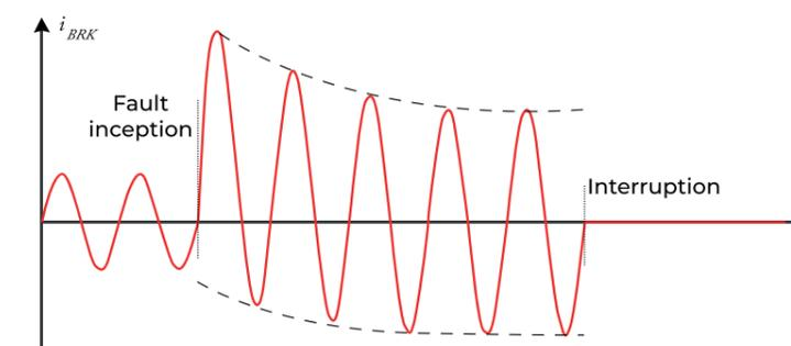
Figure 3: Graphical representation of current flowing as a result of the fault in Figure 2
