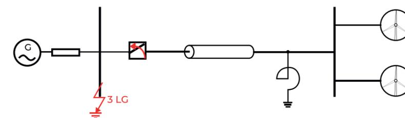
Figure 4: Circuit diagram with a shunt reactor and connected wind generation showing a fault
