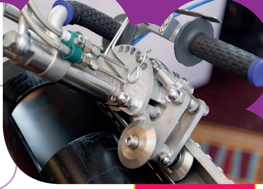
development, we have rolled out the rapid steel pipe cutters on our network and will continue using them for steel mains insertion window cutting and one-off connections of new properties.
