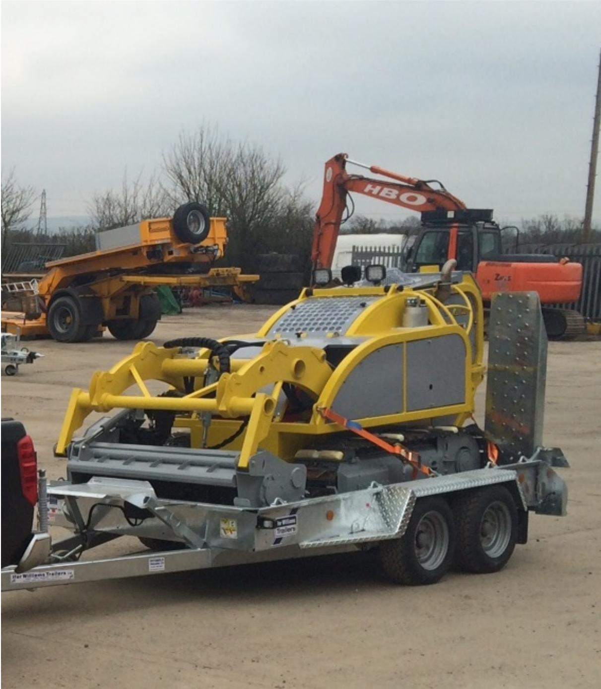
Figure 4 Remotely operated forestry mulching machine
