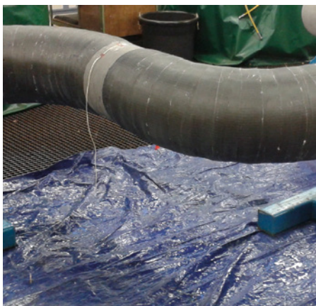
Two back-to-back bends with composite repairs applied over simulated corrosion patches, in preparation for fatigue testing.
