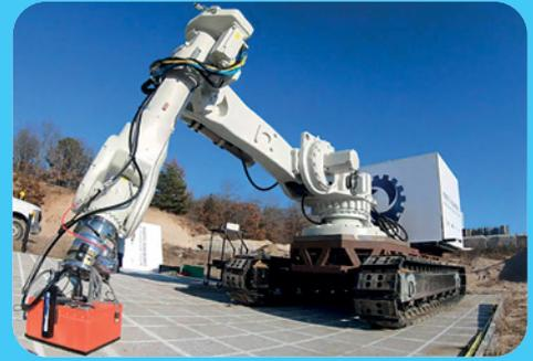
Using our mock roadway which represents a typical utility highway complete with mixed material pipeline and ducts, the team have commenced the testing of the sensor module. The results have been positive with a high accuracy of detection at various depths. More testing is to be conducted to improve accuracy of detection within different soil types.
