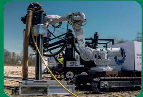
Testing has progressed with mounting the excavator head onto the robotic arm and using test beds with varying soil types including compacted hard clay. The ability to utilise the robotic arm for excavation has improved the precision in excavation operation. More testing is required to improve on the system and the process to make the excavator more robust and effective.
