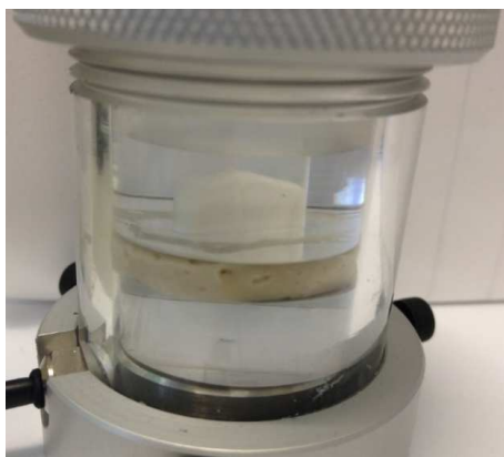
Figure 6: Repair pressure test rig to measure and visualise material response to water
