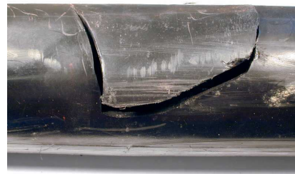
Figure 5: MV polymeric cable with typical sheath damage
