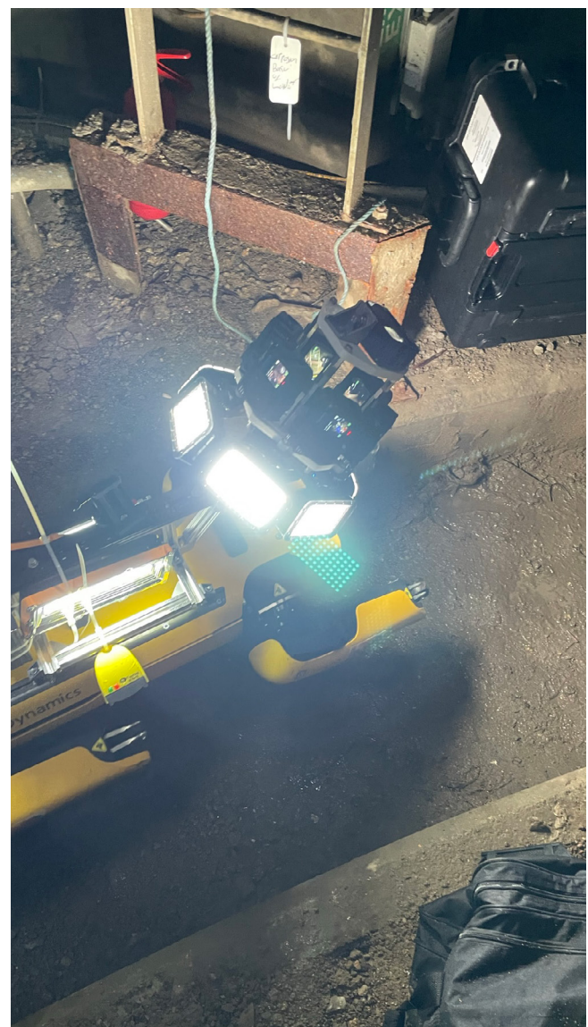
Figure 39: Boston Dynamic's Spot in action with Arup's camera module installed during phase 1.
