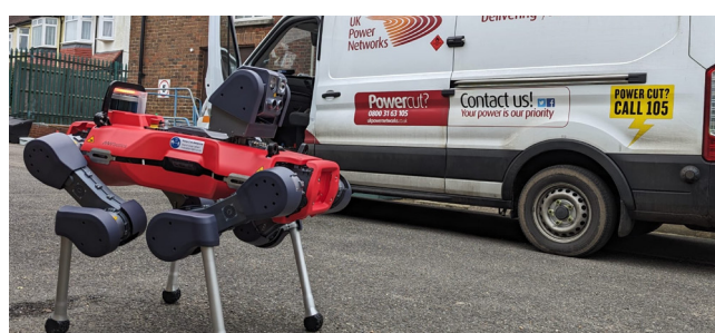
Figure 41: ANYBotics' ANYmal robot to be trialed in phase 2 for its autonomous inspection capabilities.
