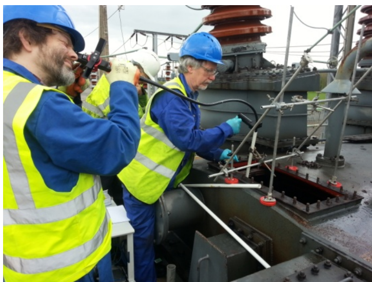
Figure 12. Trial of the intrascope probe system on a decommissioned National Grid transformer in 2014
