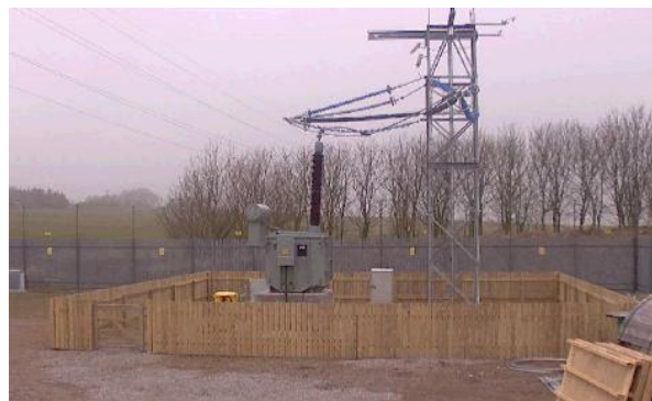
Figure 3. Installation of insulated cross arm at The Lecht (left) and St Fergus test rig (right)
