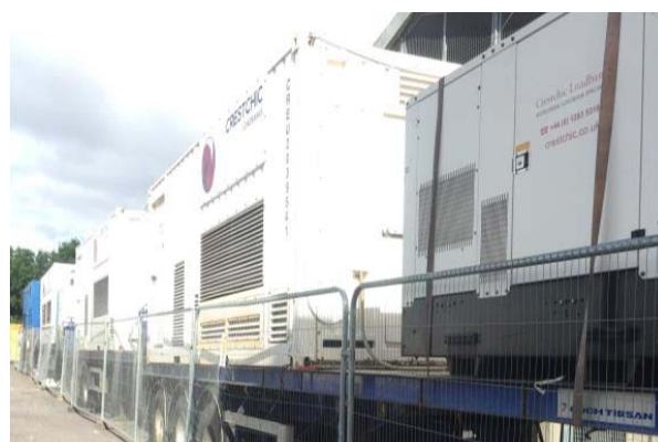
Installed Load Banks for Heat Rise Tests
