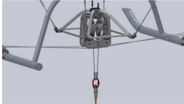
*Figure 2 - Helicopter Attachment & Release Mechanism*
