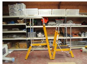
The original platform and external handrail concept was not considered a viable option due to the very poor condition of handrails at other substations in the country. It was therefore decide to go for a platform with integral handrails.
