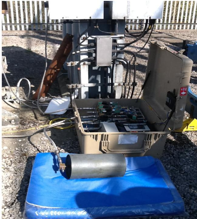
Below is a picture of the drain equipment. The hydraulic components can be seen positioned on the drum, while the electrical components are resting below.
