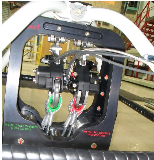
**Figure 2 – Hook attachment assembly system**
