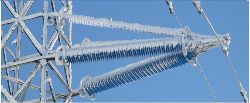
**Icing Observed On The 400kV Insulating Cross-Arm Sample In The Cairngorms**
