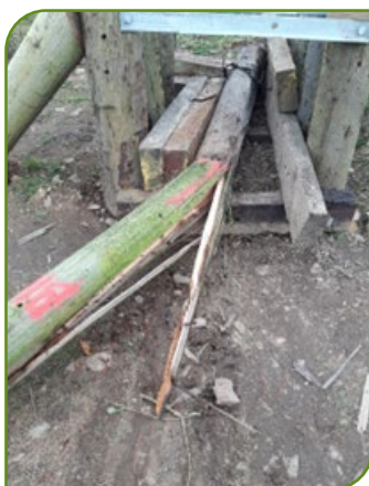
Destructive testing of a SP Energy Networks pole, showing breaking point at ground level
