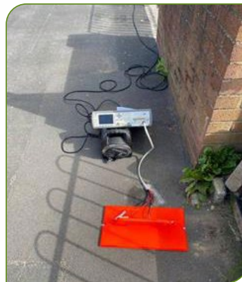
Field testing of non-intrusive device measuring thickness and air-void density of tarmac reinstatements."
