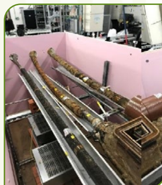
DC energisation in a lab based environment
