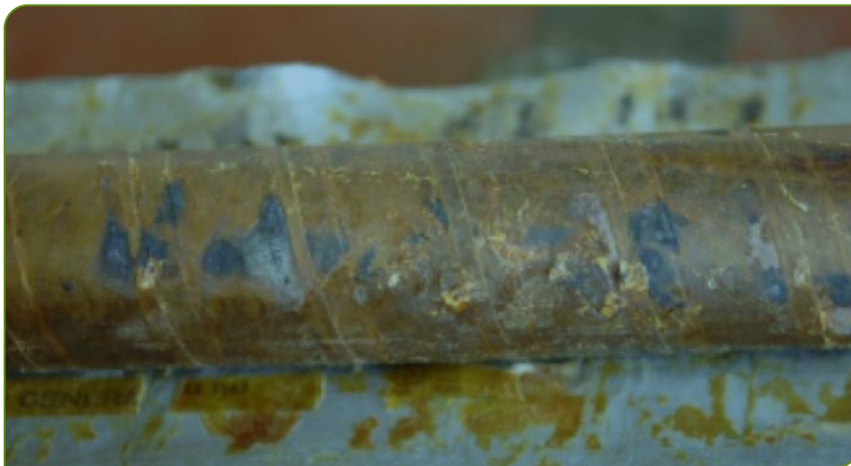
PILC cable with signs of wear and degradation
