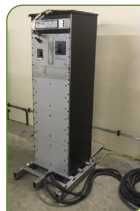
Real Time Fault level monitoring prototype
