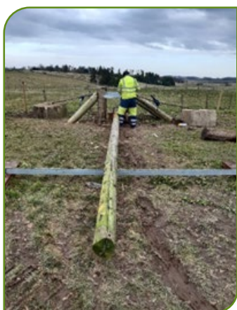
Setup of destructive testing rig in line with ASTM D1036 standard
