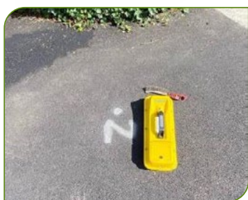
Field testing of non-intrusive device measuring thickness and air-void density of tarmac reinstatements."
