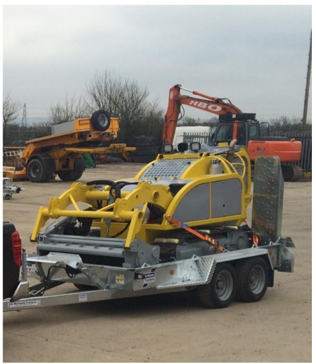
Figure 4 Remotely operated forestry mulching machine
