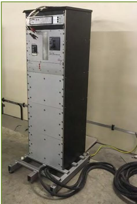
Prospective 10ms make and 90ms break currents were both measured within a 1-2% tolerance to modelled data which is very encouraging. The results were reproducible throughout testing and showed a similar tolerance in multiple network configurations. The percentage change when reconfiguring the network expected to be 10% proved to be within a 1% tolerance when compared to measured values. This is illustrated in the graphic below.
