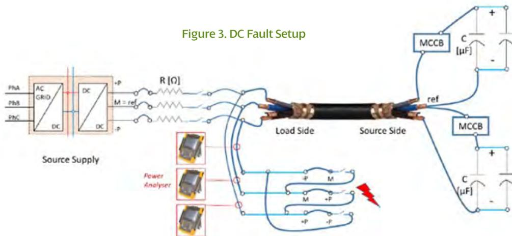
The testing programme that will be completed on each cable, joint and link box type is detailed below in figure 3.
