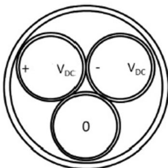
Figure 1. Three Core Bipolar Arrangement
