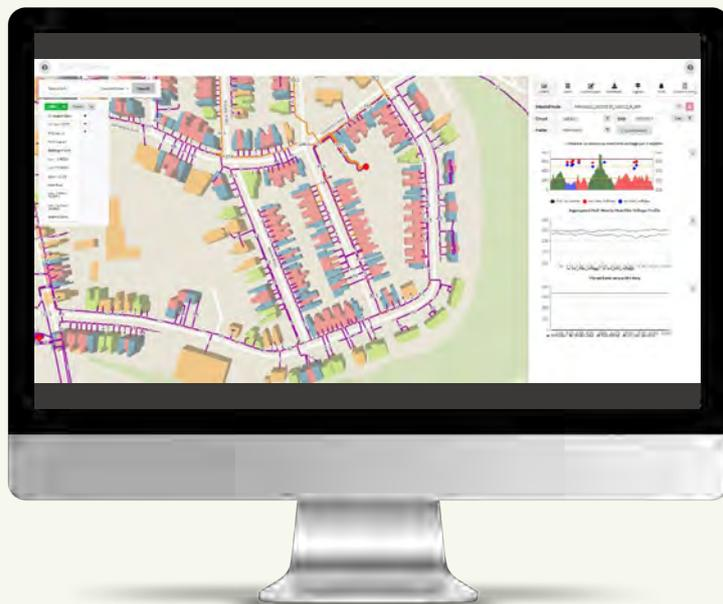
**NAVI platform visualisation showing circuit connectivity, ADMD estimation and building understanding, with Smart Meter voltage data.**
