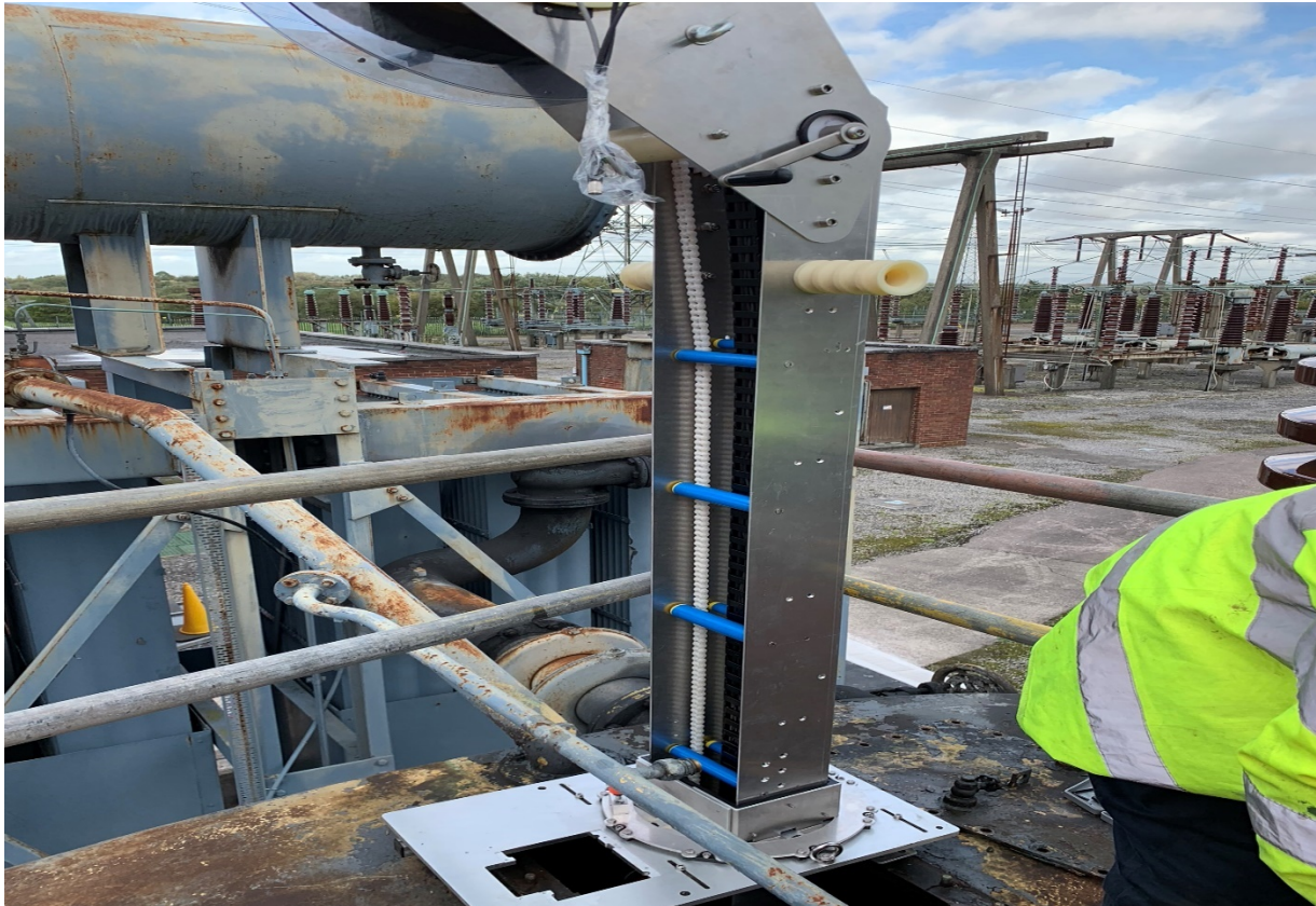
Figure 2. Accessing transformer windings with Phase 2 intrascope prototype
