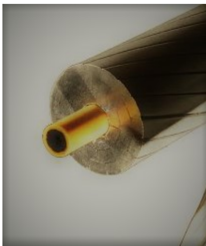
Figure 9. Cross-sectional view of the ACCC conductor
