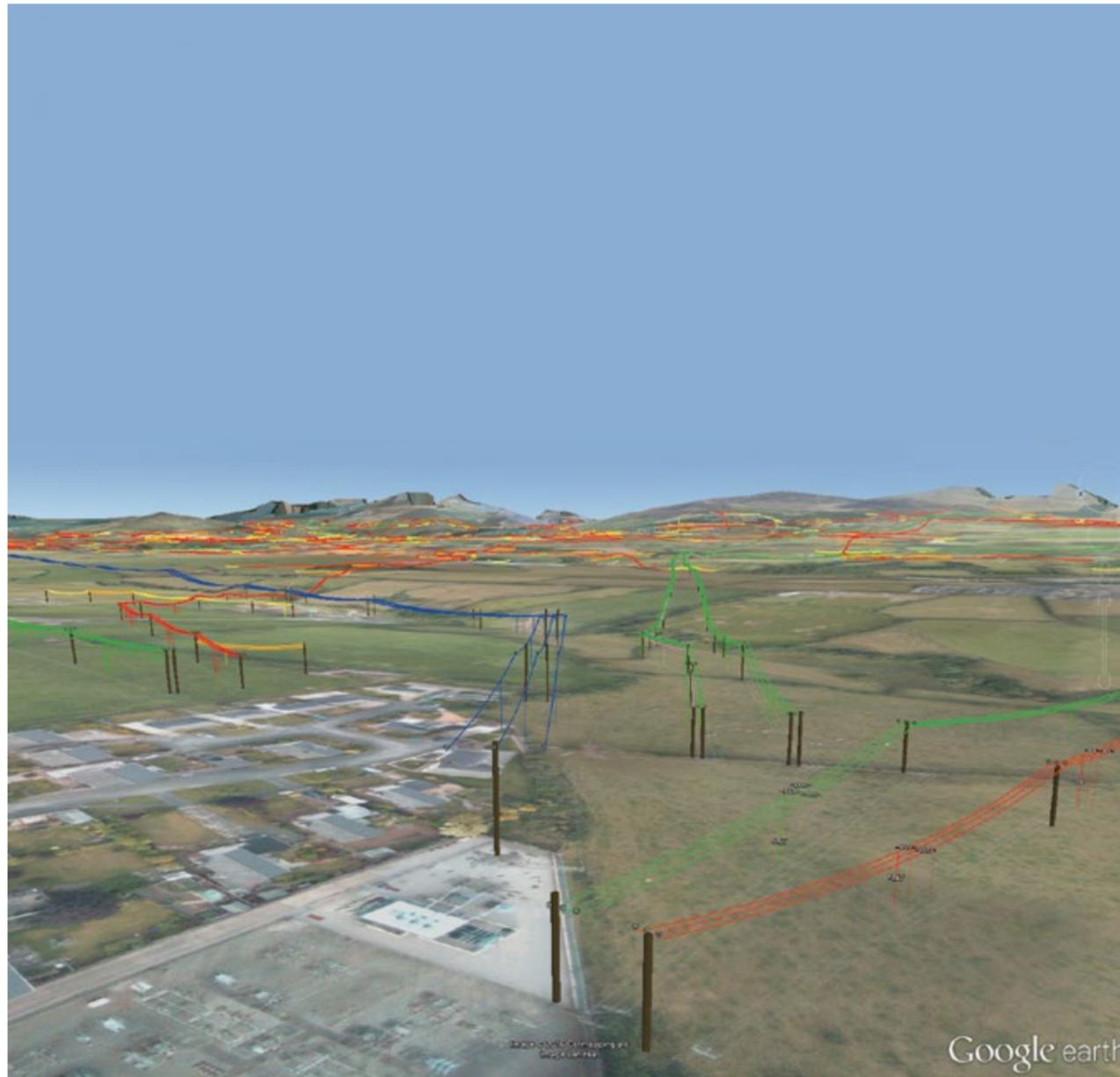
VWAM utilises Light Detecting and Ranging Technology (LiDAR) to produce a 3D model of the overhead line network. The network is captured using a fixed wing aircraft which blanket covers the distribution network. The raw LiDAR data collected is processed using a patented algorithm to produce a detailed analytic spreadsheet and 3D visualisation.
