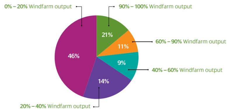
Figure 10 – The probability of the windfarm output being in different level of maximum capacity, a 15 month period has been considered
