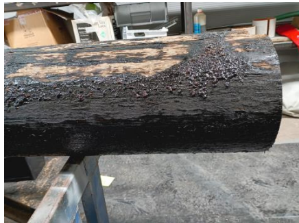
Creosote deposit post extraction
