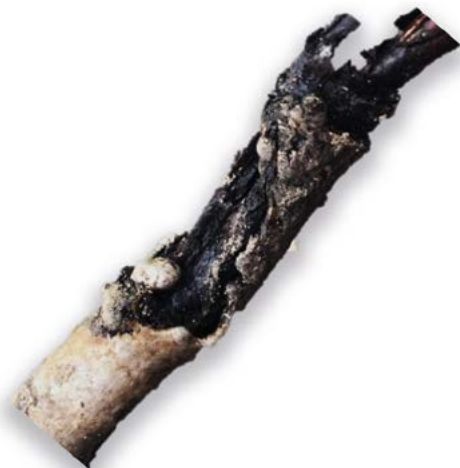
Faulted cable found during a MAAV survey and replaced
