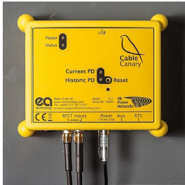
Cable Canary device that monitors vertical transition joints within substation using partial discharged techniques
