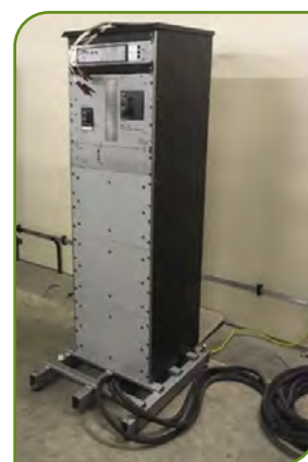
Real Time Fault level monitoring prototype
