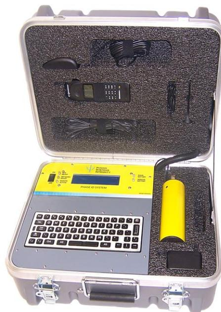
**Figure 2.1 Phase ID Field Unit Model 1500**
