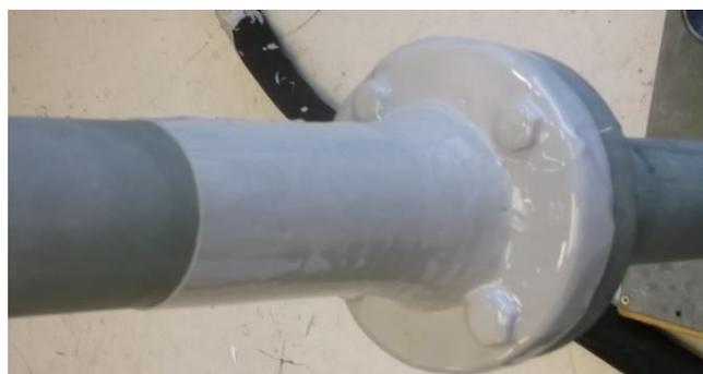
**Figure 5.2: Oxifree coating applied to a leaking section of pipe.**
