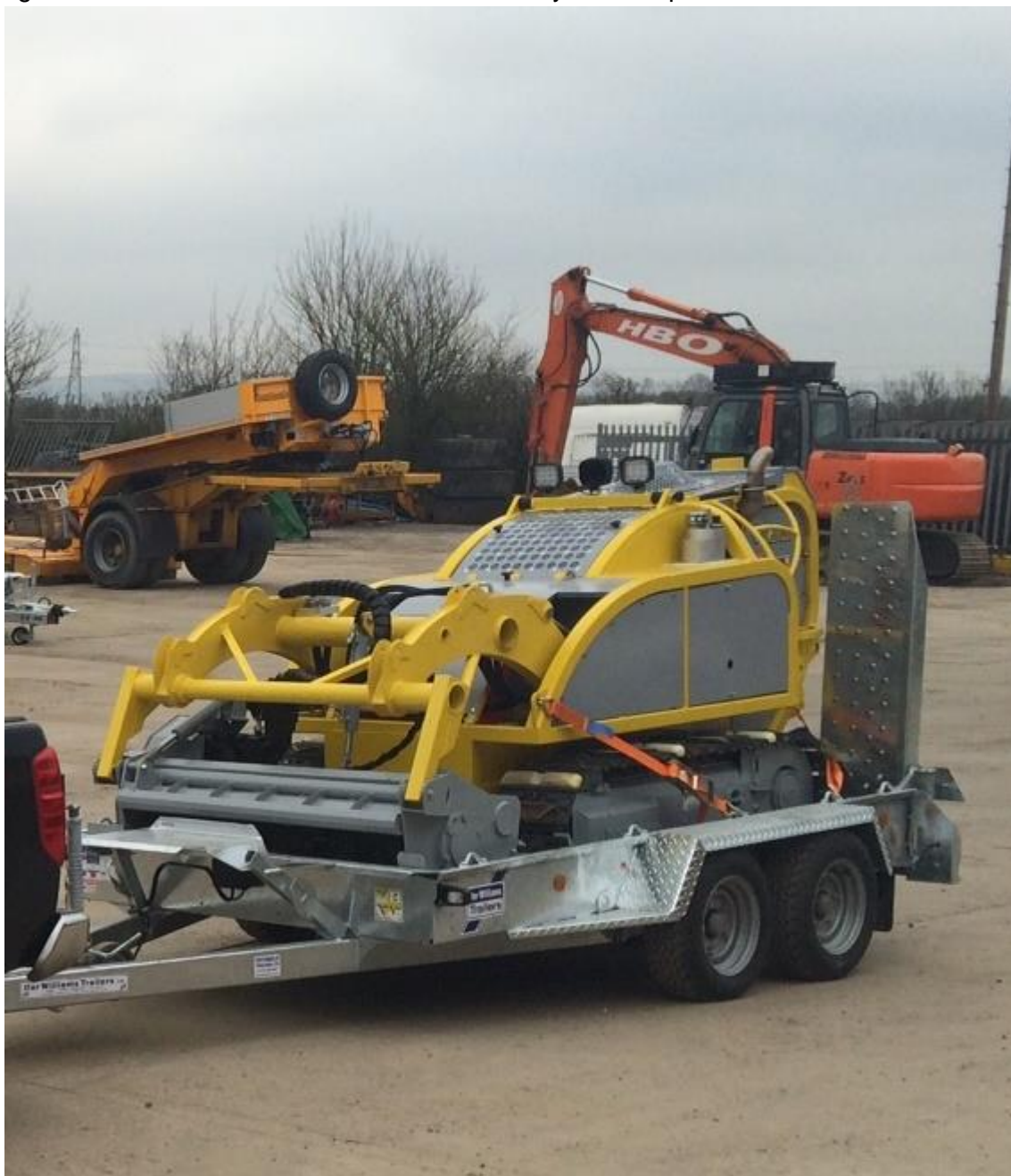
Fig 4. Remotely operated forestry mulching machine
