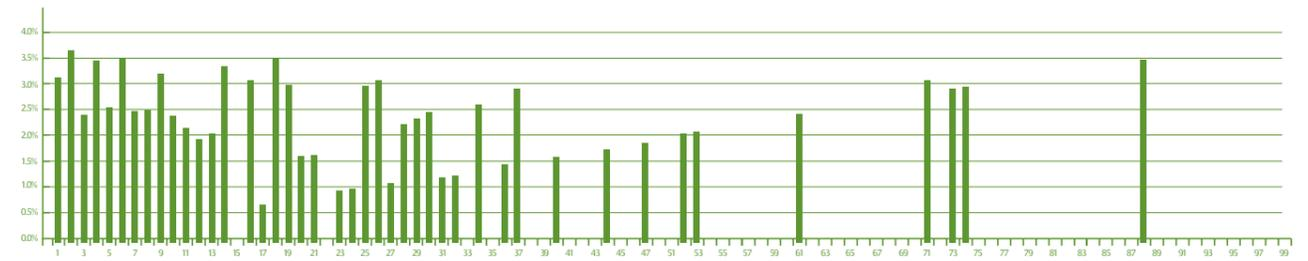
Figure 11 – The probability of the windfarm outputs stays on > 90% of maximum capacity for consecutive hours
