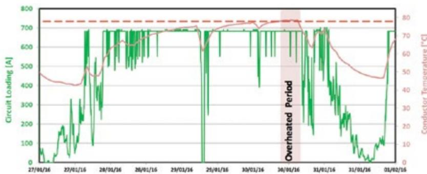
Figure 9 – The wind farm output and the cable conductor temperature variations when the output of windfarm is increased to 39 MW (simulation) – Dotted line shows the permissible temperature limit
