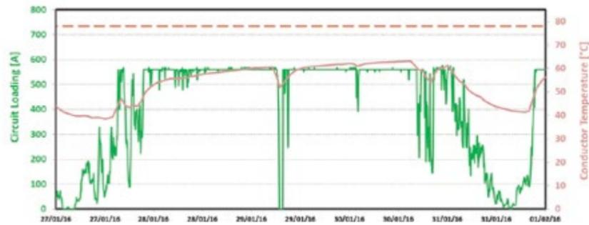
Figure 8 – The wind farm output and the cable conductor temperature variations when the output of windfarm is limited to 32 MW – Dotted line shows the 78°C permissible temperature limit
