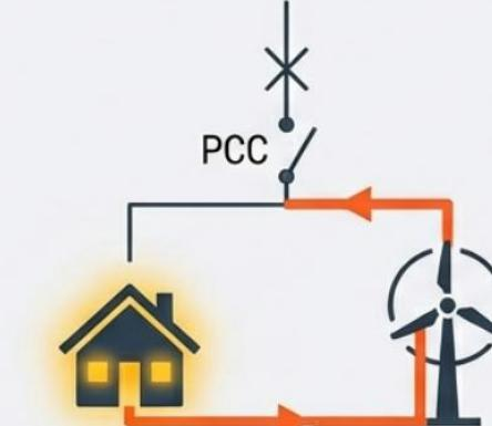
**Resilient.** System detects fault, opens Point of Common Coupling (PCC), and balances local Generation & Demand. Lights stay on.
