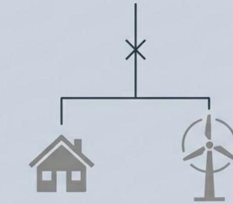
**Disrupted.** Loss of Mains protection trips all generation. Customers go dark. Circuit remains de-energised for safety.
