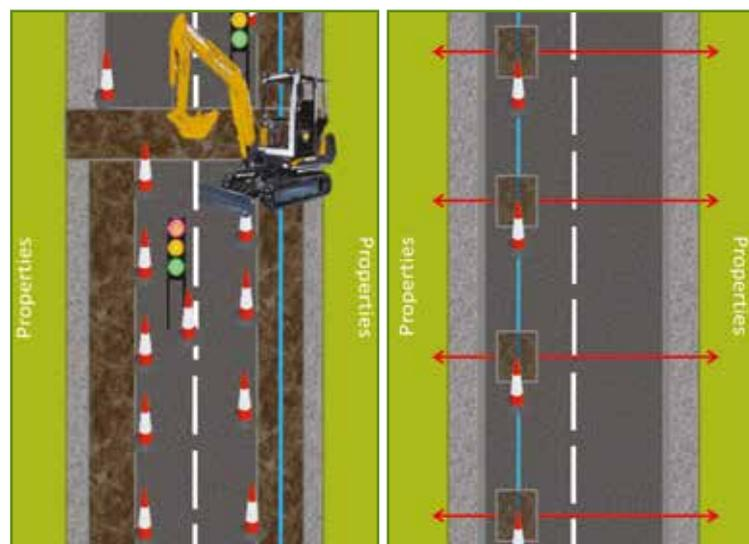
**The above diagram outlines the potential difference between the traditional method with road crossing and traffic management vs. the Mini Mole method with no open excavation road crossings and limited excavation requirements.**
