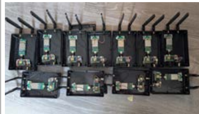
Figure 6: Prototype mobile network monitoring devices which were deployed at UK Power Networks sites
