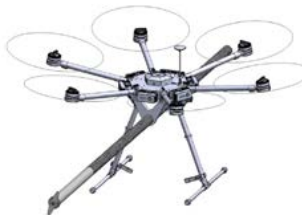
Figure 16: Option 1 retrofit of a commercially available 6 rotor drone (computer aided design model)
